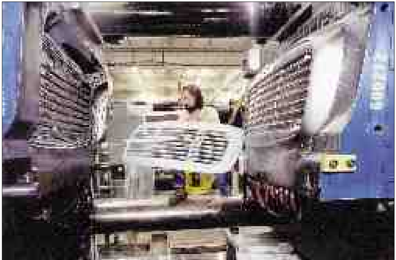
A new 3000-ton injection molding press allows Guardian Morehead to manufacture larger parts, such as grilles, fascias and body panels.
