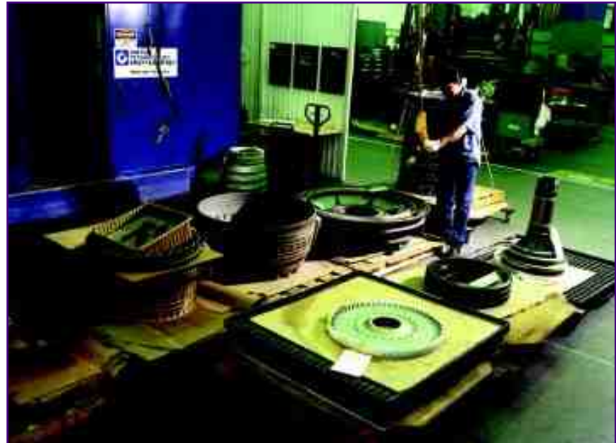
This photo illustrates the wide variety of parts that an airline overhaul facility handles. These parts will be cleaned in the large parts washer (blue cabinet in background).
