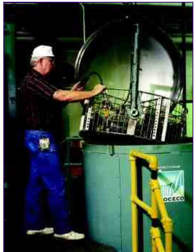
Parts removed from the components parts washer are loaded into the vacuum dryer.
