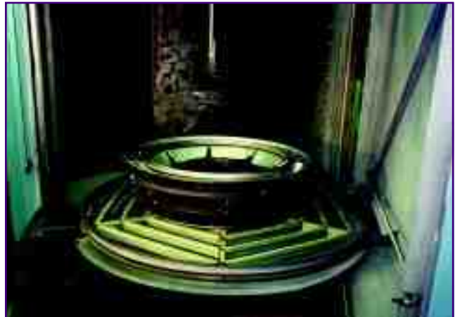
This close-up of a large jet engine mid-frame case shows the washer's center nozzle lance. This nozzle permits the cleaning of interior surfaces of cylindrically shaped components.
