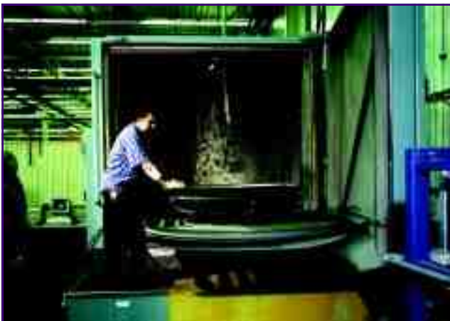
A jet engine mid-frame case is loaded into the large parts washer.
