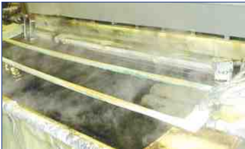
The predominant cleaning methods are still done by immersing parts in solution.
