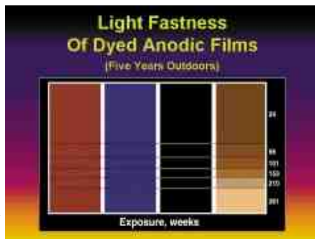
Fig. 2—Dyed anodic coatings, after five years of exposure to sunlight (Kingston, Canada), illustrate lightfastness of selected dyes. Bottoms - continuously exposed; Tops - shielded from sunlight.
