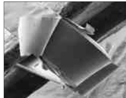
Fig. 2—SEM photo of typical adhesion failure. After heating, the SnPb deposit separates cleanly from the Cu substrate, exposing a dark-colored interface.
