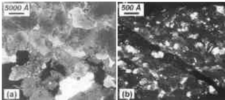
Fig. 3—TEM dark field images of (a) conformable and (b) typical nickel coatings showing different grain sizes.
