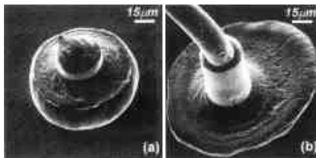
Fig. 5—SEM images showing ball bonds after pull test. Wire bonding at 180°C under (a) appropriate and (b) excessive force and power.
