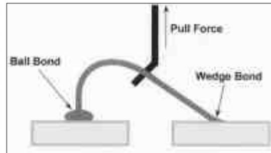
Fig. 4—Schematic gold wire bonding and pull test.
