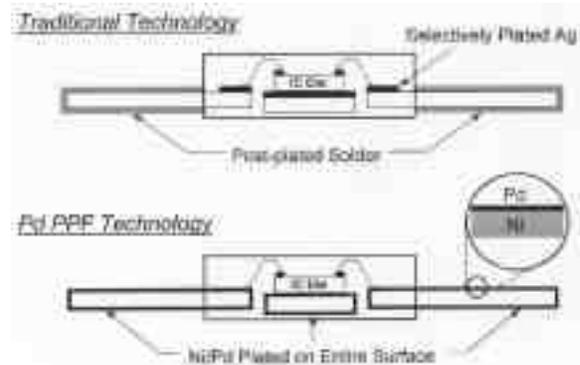
Fig. 1—Schematic cross sections of the leadframes plated with silver and solder or nickel/palladium, after die attach, wirebonding and encapsulation and before trimming-and-forming.
