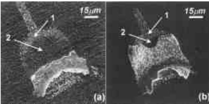
Fig. 7—SEM images showing broken wedge bonds made at (a) 100°C and (b) 180°C after pull test.
