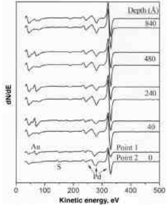
Fig. 8—AES spectra showing a typical surface composition at the perimeter (point 1) and inner part (point 2) of a broken wedge bond at different sputtering depths.
