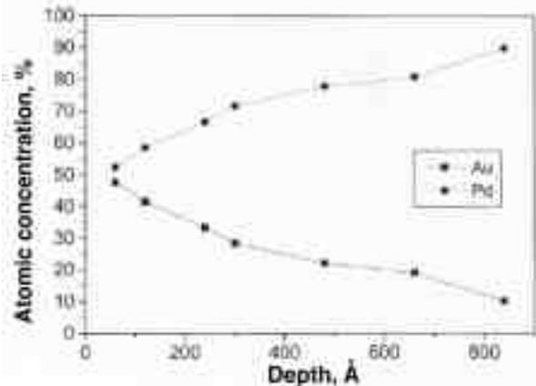
Fig. 9—A typical AES depth profile at the perimeter of a broken wedge bond.
