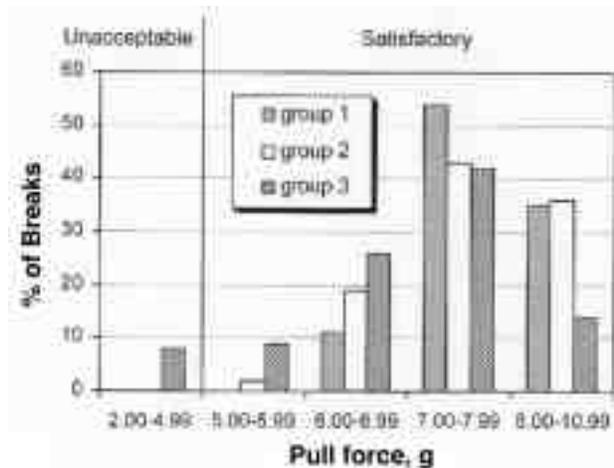
Fig. 11—Distribution of wirebonding breaks within different pull force ranges using the different palladium finishes.
