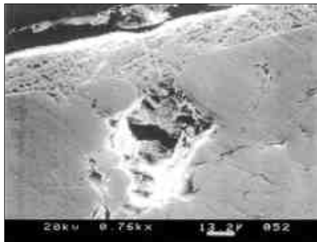
Fig. 4— Cross section of porous substrate.
