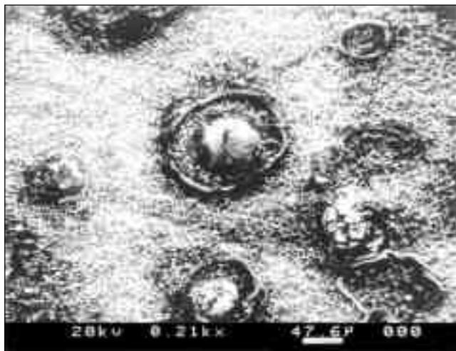
Fig. 1—Bleed-out on over-etched aluminum after lifting blister.
