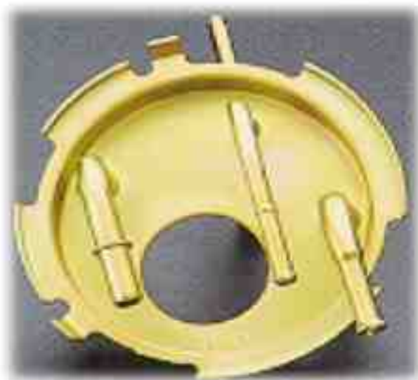
Stampings such as this one are formed by the shearing action of a sharp-cutting die against a sheet of metal. Stampings are relatively easy to prepare for plating, because they usually have only cutting oils on the surface, and the metal is not significantly deformed by the operation.
