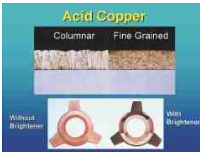
This shows the dramatic effect of the addition agent in producing a highly reflective bright deposit. In the absence of the addition agent, the deposit is dull and salmon in color. One of the unique features of the bright acid copper process is the ability to plate and fill in grooves occurring from polishing. Result: The deposit is smoother than the basis metal.
