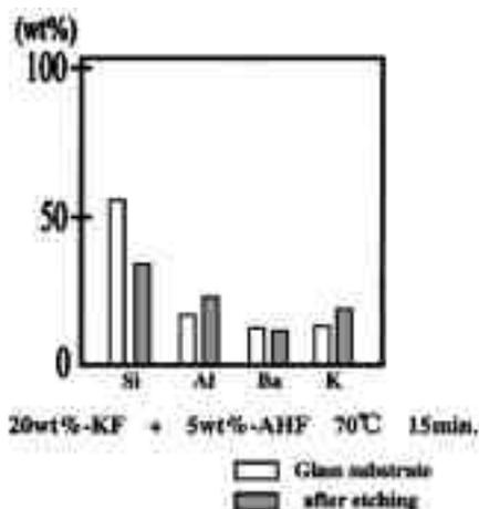
Fig. 5—EDS analysis results for the glass surfaces.
