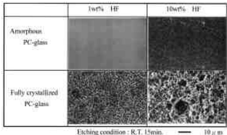
Fig. 3—SEM images of the PC glass surfaces.
