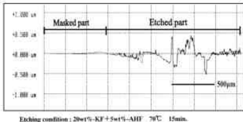
Fig. 6—Surface roughness measurements on amorphous PC glass after etching.
