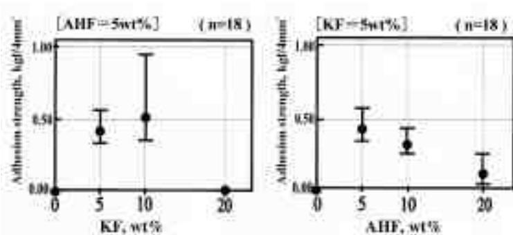
Fig. 8—Effect of each etching composition on adhesion strength on amorphous PC glass.
