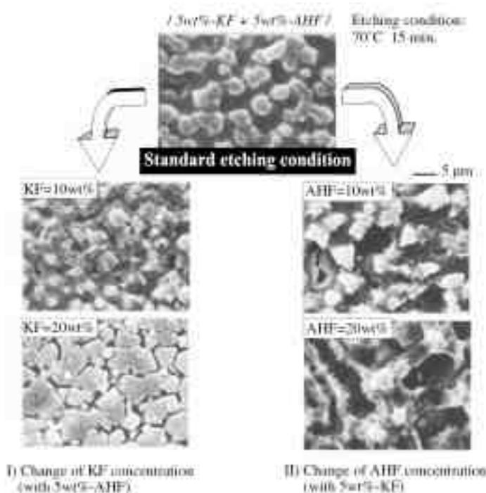
Fig. 4—Relationship between the etchant composition and the surface morphology on amorphous PC glass.
