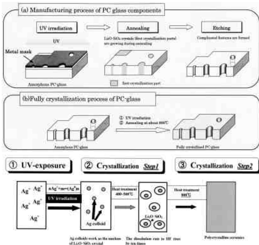
Fig. 1—Crystallization process for PC glass.
