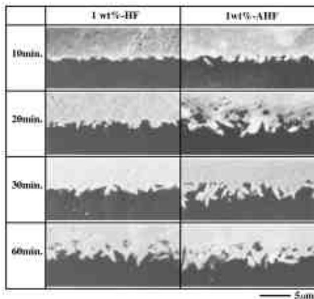
Fig. 11—SEM images of cross sections for fully crystallized PC glass.
