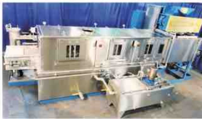
This belt spray system is configured for wash, rinse, rust inhibit, recirculating hot air dryer, oil coalescer, and wash filtration.
