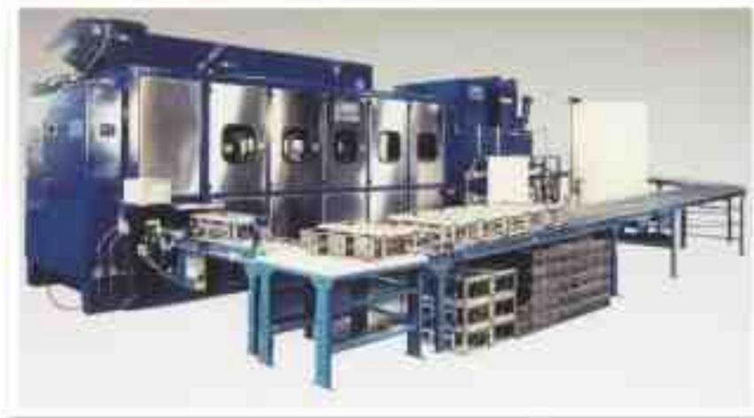
A five-tank vertical agitation and rotation system with material handling and closed-loop wastewater treatment system. It utilizes a wash, ultrasonic wash, three counterflow rinses, and rotation of baskets in a recirculation hot air dryer.
