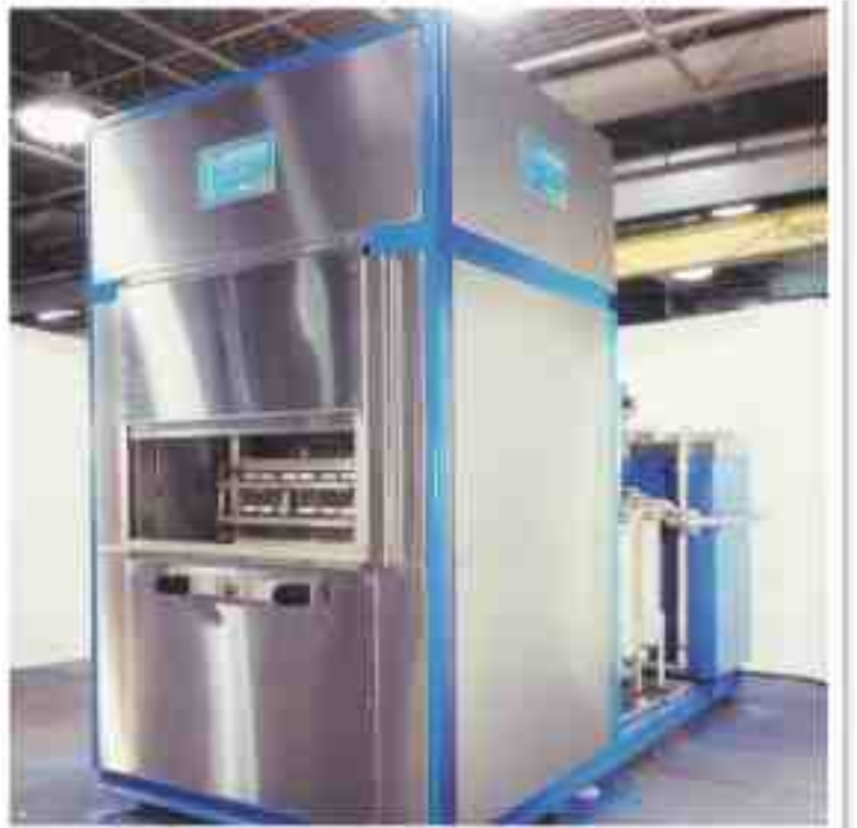
Cellular vertical agitation and rotation system that accepts up to six baskets approximately 12 in. x 18 in. x 6 in., for a total work envelope of 36 in. x 18 in. by 12 in. The system is configured for wash, rinse and dry.
