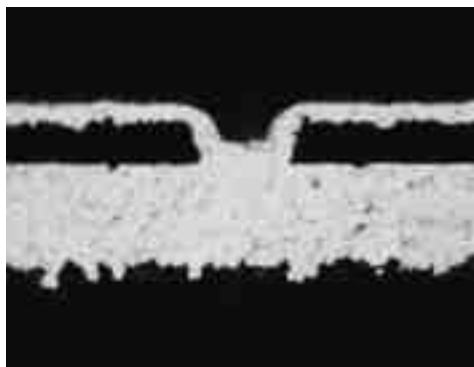
Fig. 11—Electrically mediated plating of 30 mm microvia for CSP.
