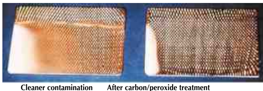
Figure 4—Effect of proprietary cleaner contamination.
