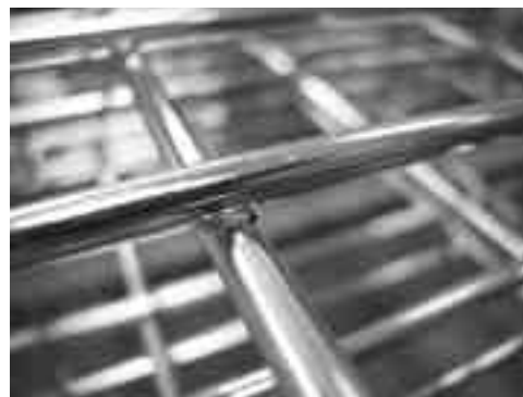
Nodules produced by welding.
