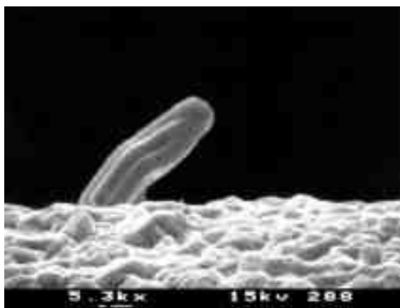
Fig. 8—Tin whiskers observed on Deposit III.
