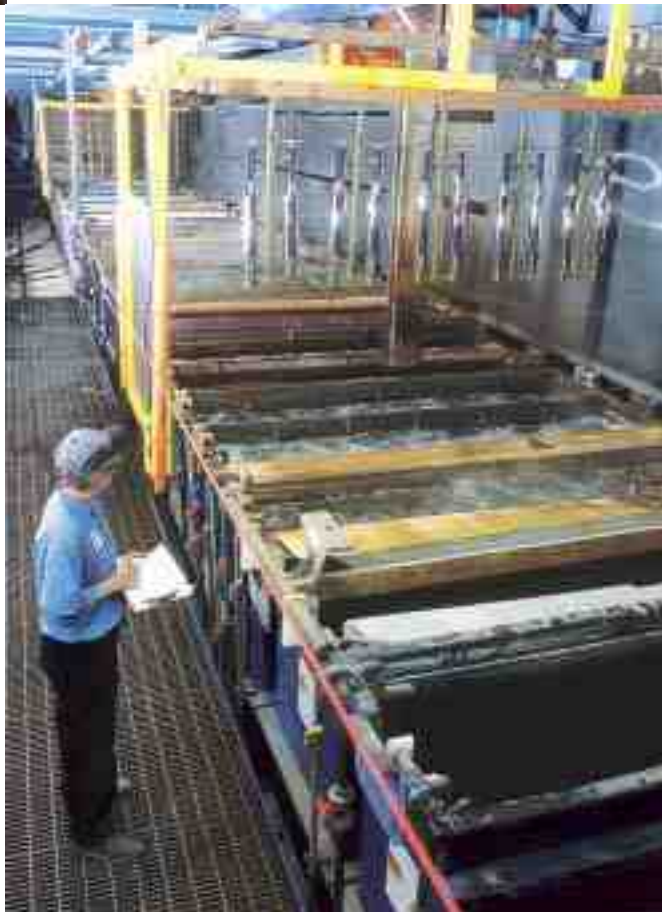
Plating lines are monitored constantly to ensure that parts are receiving the proper finish.
