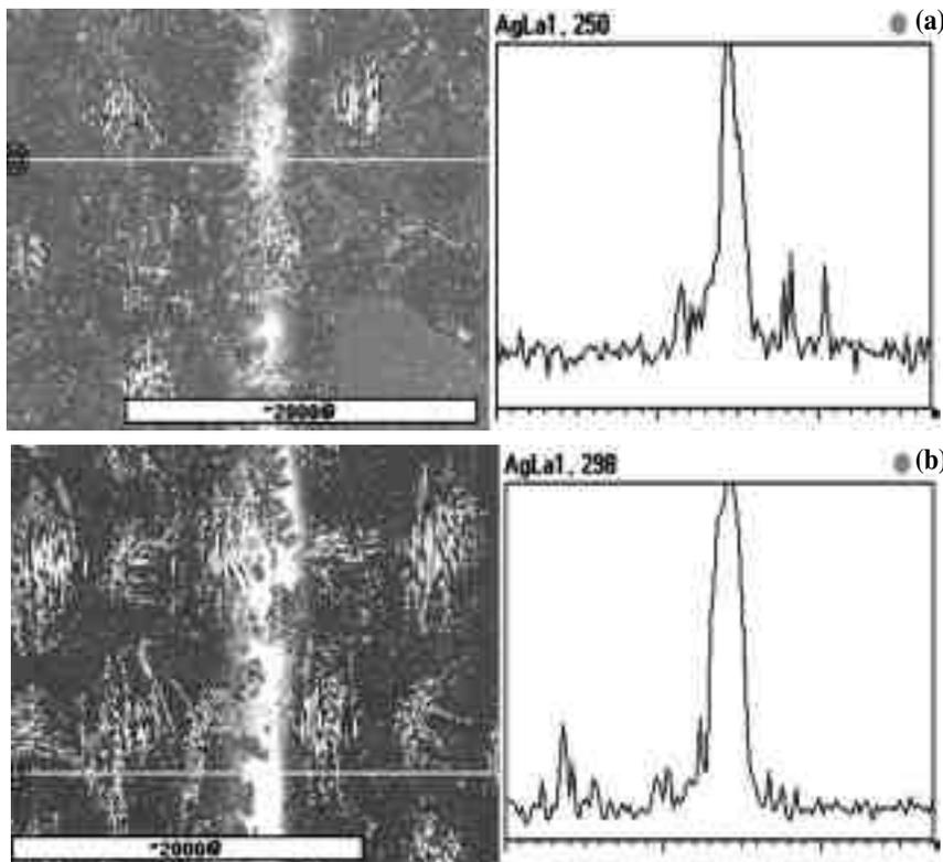
Fig. 5—Line analysis of EPMA for silver layers deposited on the substrate with different laser power levels: (a) 2.5 W; length, 2.696 mm; width, 0.25 mm. (b) 3.5 W; length, 2.717 mm; width, 0.35 mm.
