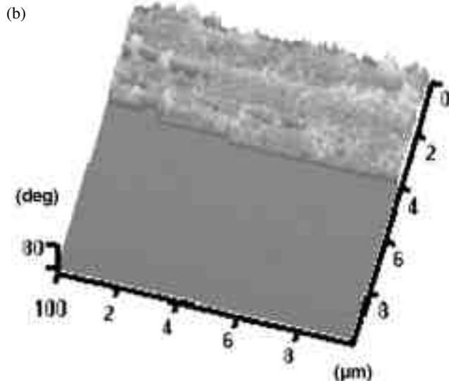
Fig. 11—DFM three-dimensional images of the silver layer: (a) surface morphology images; (b) phase images. The laser power was 4.0 W and the scanning velocity was 0.4 m/min.
