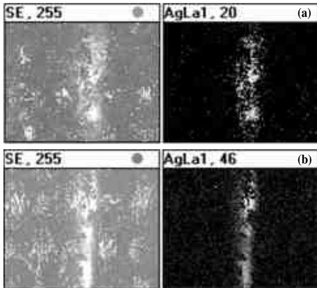
Fig. 3—Morphology of the silver layer deposited on the surface of epoxy resin at (a) 2.5 W and (b) 3.5 W laser power.
