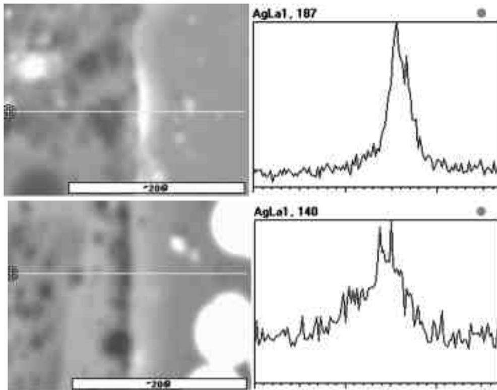
Fig. 10—Thickness of metal layers deposited on epoxy resin board at different solution concentrations:
