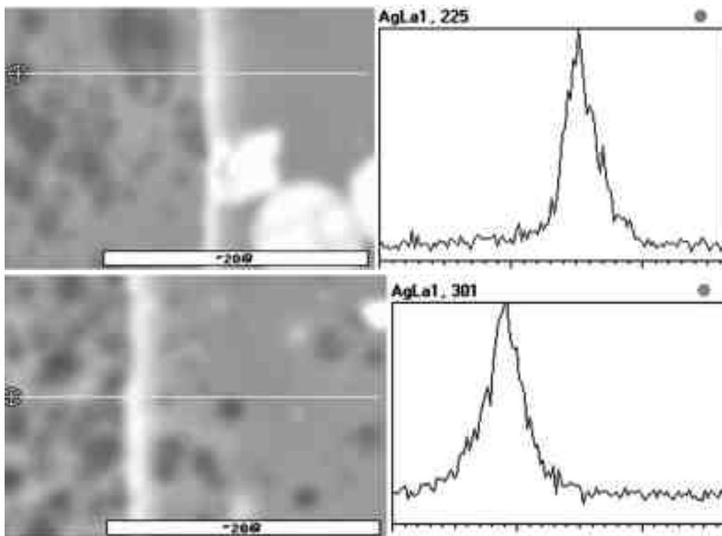
Fig. 8—Transverse section line analysis of EPMA of metal layer thicknesses at different laser power levels: (a) 3.0 W; length, 26.96  $\mu\text{m}$ ; thickness, 5  $\mu\text{m}$ . (b) 4.0 W; length, 26.96  $\mu\text{m}$ ; thickness, 7  $\mu\text{m}$ .
