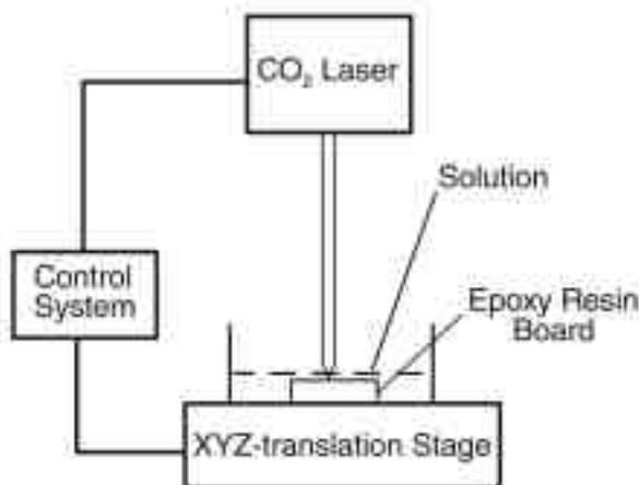
Fig. 1—Setup for CO<sub>2</sub> laser-induced deposition from aqueous solution.
