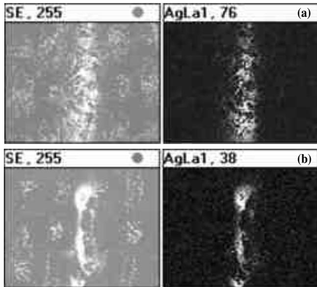
Fig. 4—Morphology of the silver layer deposited with (a) 1 mm and (b) 2 mm thickness of liquid film on the epoxy resin board.
