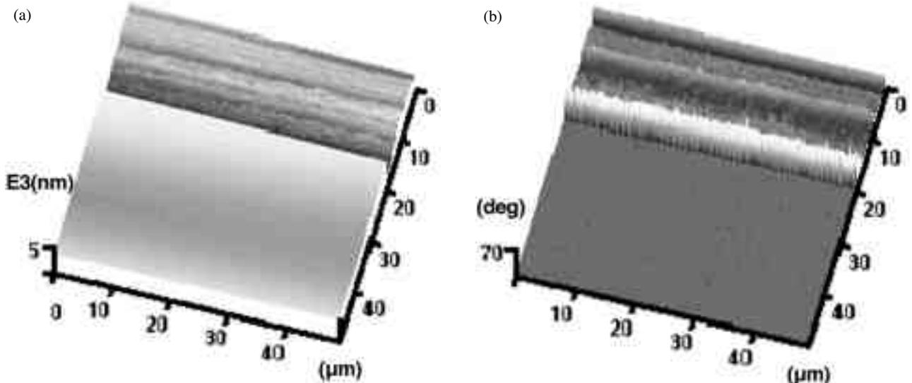
Fig. 12—DFM three-dimensional images of copper layer on the silver layer: (a) surface morphology images; (b) phase images. The copper layer was deposited on silver by electroless plating. The solution composition was 0.1M  $\text{CuSO}_4$ , 0.2M NaK-tartrate, 0.1M NaOH and 6M HCOH.
