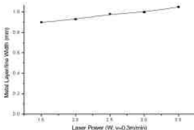
Fig. 7—Influence of the laser power on the width of the metal layer/line.
