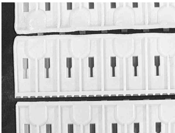
Figure 8—Metral headers showing results of reflow: bottom part, 223°C (433°F); middle part, 262°C (504°F) and top part, 272°C (522°F) board temperatures, respectively. Parts are made from liquid crystalline polymer (LCP) with a melting point of 280°C (536°F).
