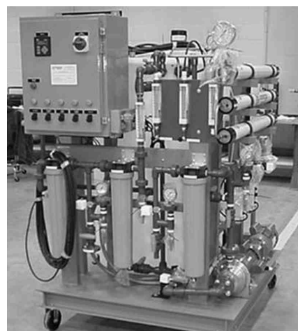
Figure 6—Onsite pilot setups for (a) microfiltration and (b) reverse osmosis evaluations.
