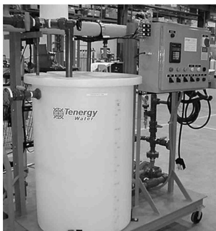
Figure 6—Onsite pilot setups for (a) microfiltration and (b) reverse osmosis evaluations.
