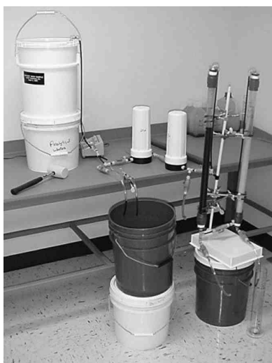
Figure 5—Laboratory study setup for evaluating ion exchange as a removal process.
