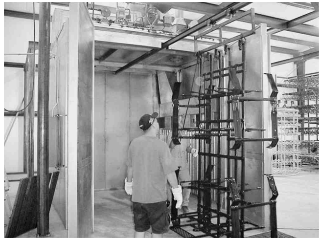
Fig. 8—Curing of plastisol in oven. 5
