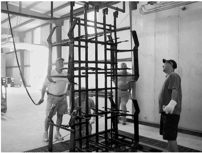
Fig. 7—Plastisol dipping of plating rack 5 .
