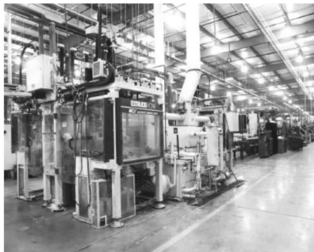
Fig. 12—Electrolytic machining equipment processing airbag housings.
