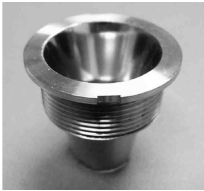
Fig. 15—Internal surface polishing by electrolytic material removal.
