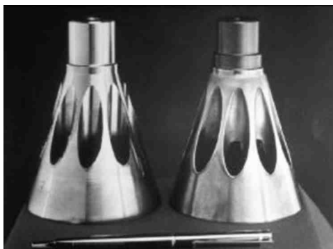
Fig. 13—Cone with electrolytically formed edges.
