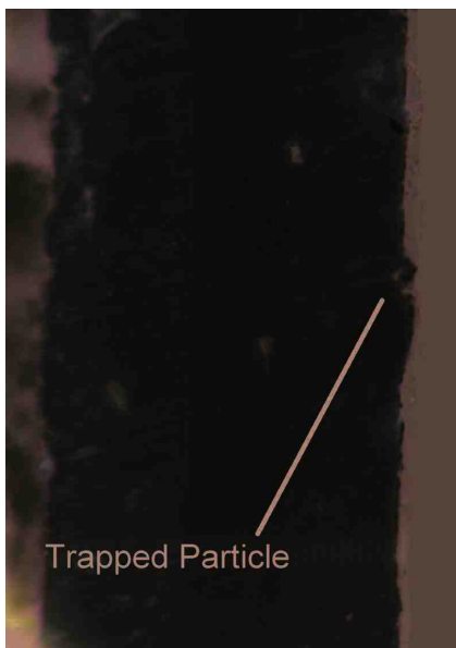
Photo 3—Cross section showing trapped particle.
