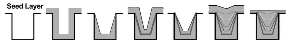
Fig. 5—Novel filling profile for electrically-mediated process. The first picture shows the initial seed layer. This is followed by the conformal deposition of copper. Next the preferential etching of the upper sidewalls and re-entrant of interconnect feature is shown. The final result is a void-free copper filled feature with minimal overfill and a planarized surface.
