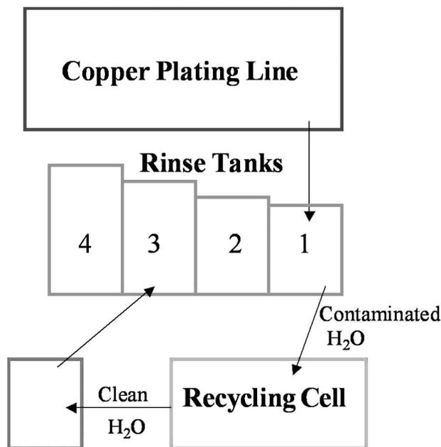
Fig. 9—Schematic diagram of the in-house copper-plating line with recycling in treatment mode.
