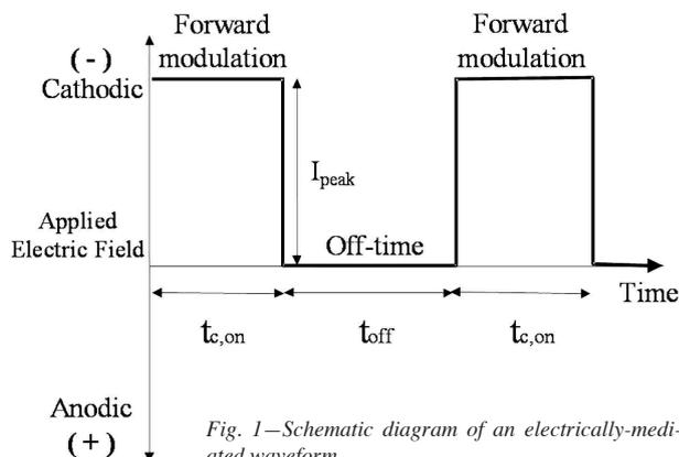
Fig. 1—Schematic diagram of an electrically-mediated waveform.
