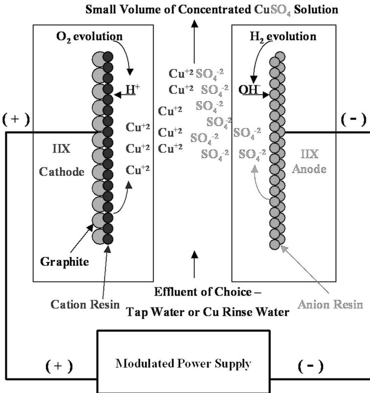
Fig. 4—Schematic diagram of cell regeneration.
