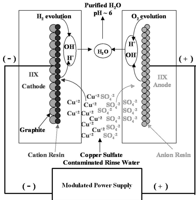
Fig. 3—Schematic diagram of the in-process recycling unit for the treatment of copper-plating rinse water.
