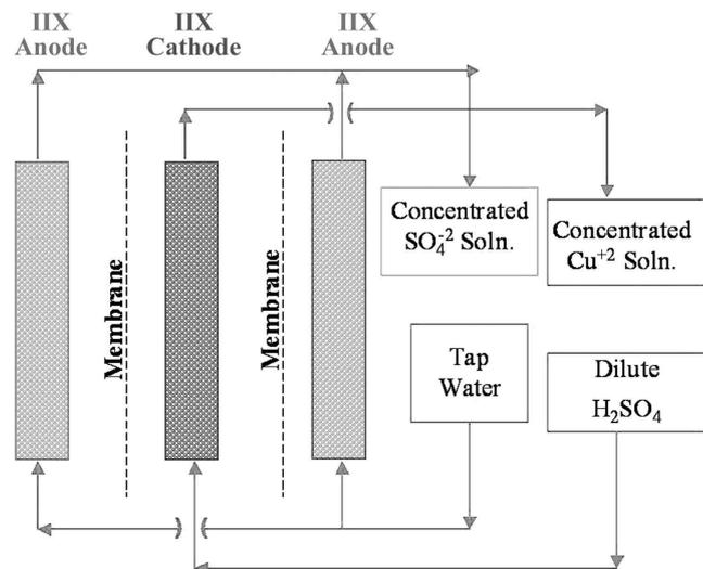
Fig. 6—Flow schematic diagram for cell regeneration.
