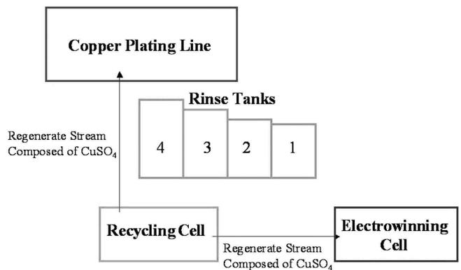
Fig. 10—Schematic diagram of the in-house copper plating line recycling system in regeneration mode.
