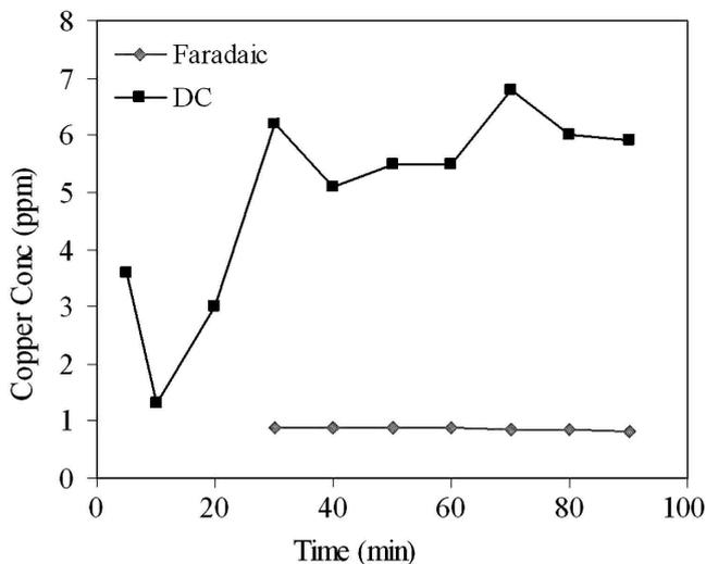
Fig. 7—Effect of the electrically-mediated process on copper removal as compared with DC treatment.
