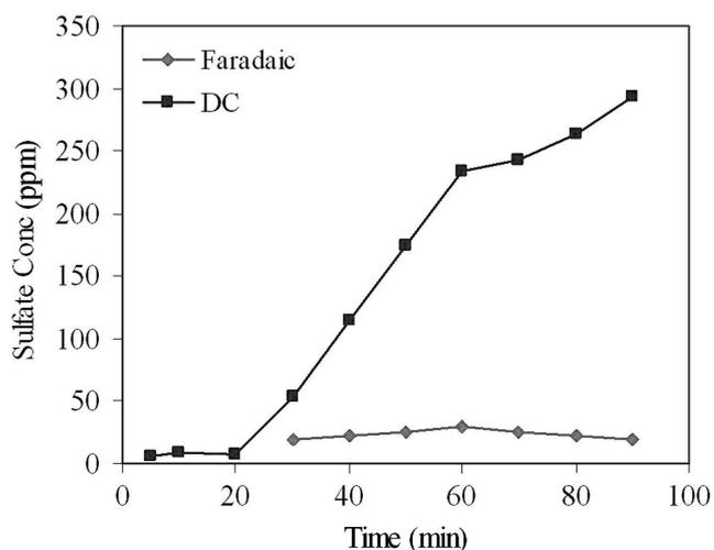
Fig. 8—Effect of the electrically-mediated process on treatment as compared to DC treatment.
