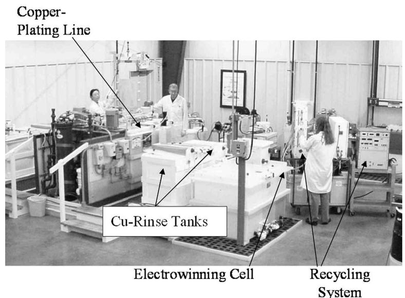
Fig. 11—Photo of the in-house copper plating line including an in-process recycling system.
