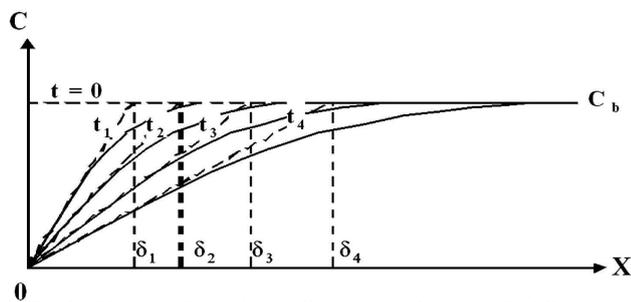
Fig. 2—Mass transfer in electrically-mediated electrolysis by diffusion.
