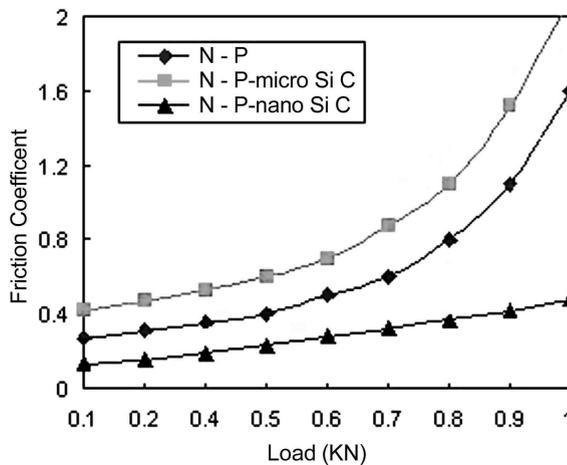
Fig. 2—Dependence of friction coefficient on load.
