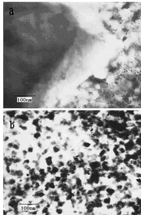
Fig. 6—The structure of (a) Ni-P/micro-SiC coating and (b) Ni-P/nano-SiC coating.
