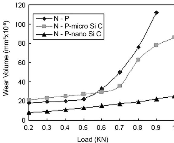
Fig. 1—Dependence of wear volume on load.
