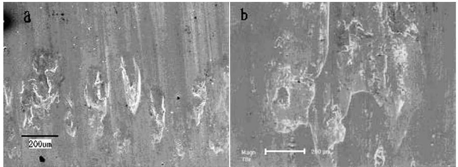
Fig. 4—The sticking friction mark of (a) Ni-P/nano-SiC coating and (b) Ni-P/micro-SiC coating.
