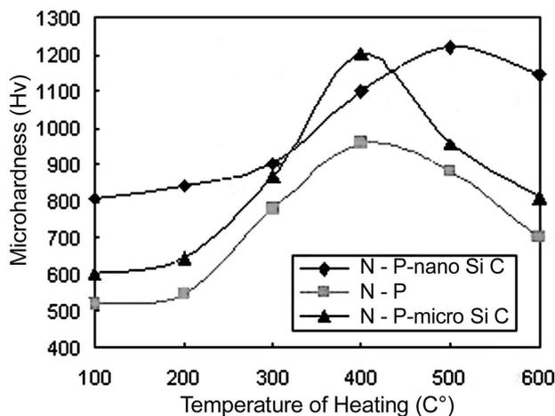
Fig. 5—Hardness vs. heating temperature.
