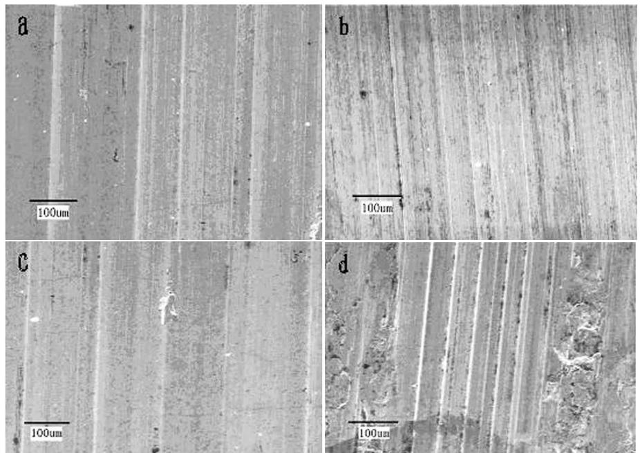
Fig. 3—The wear scar of (a) Ni-P/nano-SiC coating under 0.5 kN load; (b) Ni-P/micro-SiC coating under 0.5 kN load; (c) Ni-P/nano-SiC coating under 0.8 kN load; (d) Ni-P/micro-SiC coating under 0.8 kN load.
