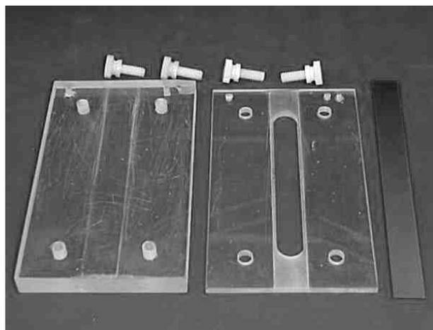
Figure 3—Plating block disassembled.
