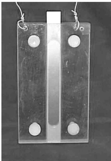
Figure 2—Plating block and strip.
