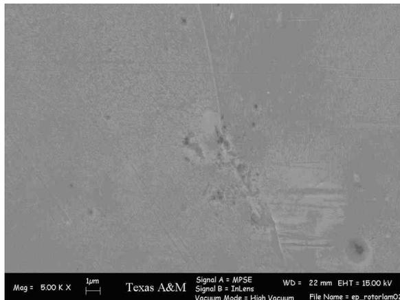
Figure 7—A 5000X view of the final electropolished surface.
