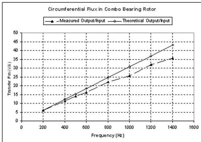
Figure 2—Frequency response from circumferential flux in an unelectropolished rotor.
