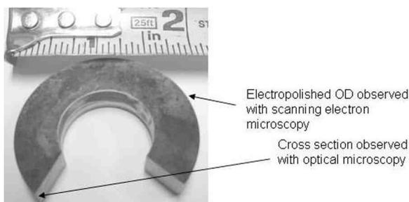
Figure 3—Electropolished rotor laminate stack.
