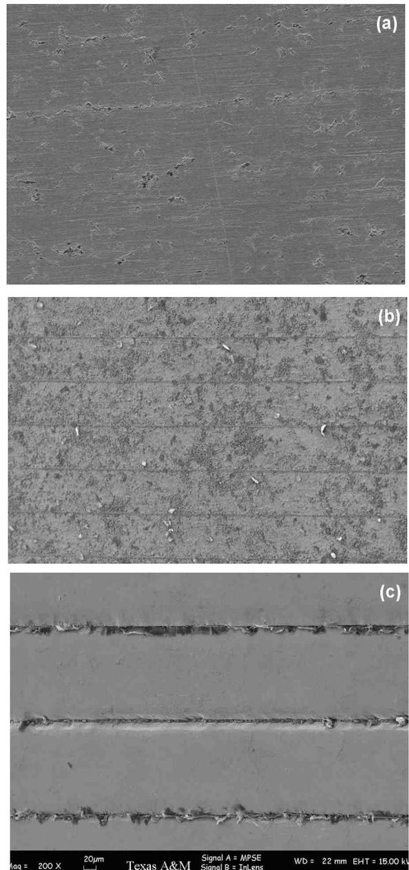
Figure 5—Scanning electron micrographs of the rotor OD: (a) The rotor lamination OD after grinding; (b) After polishing with electrolyte containing sulfuric acid; (c) After polishing with electrolyte containing ethylene glycol and hydroxyacetic acid.
