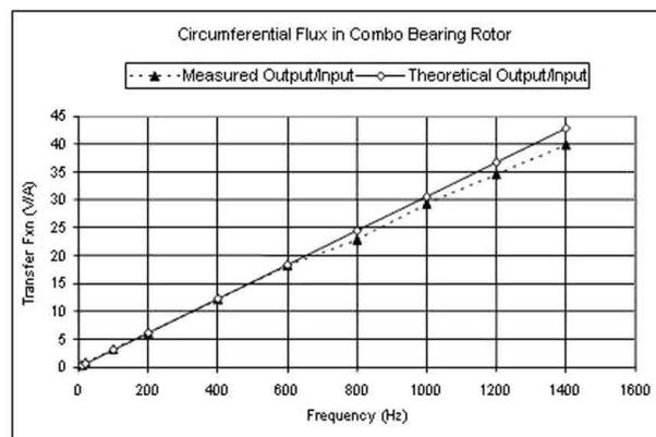
Figure 8—Frequency response from circumferential flux in an electropolished rotor.
