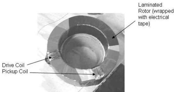
Figure 1—Experimental setup for measuring effects of eddy currents in a rotor.
