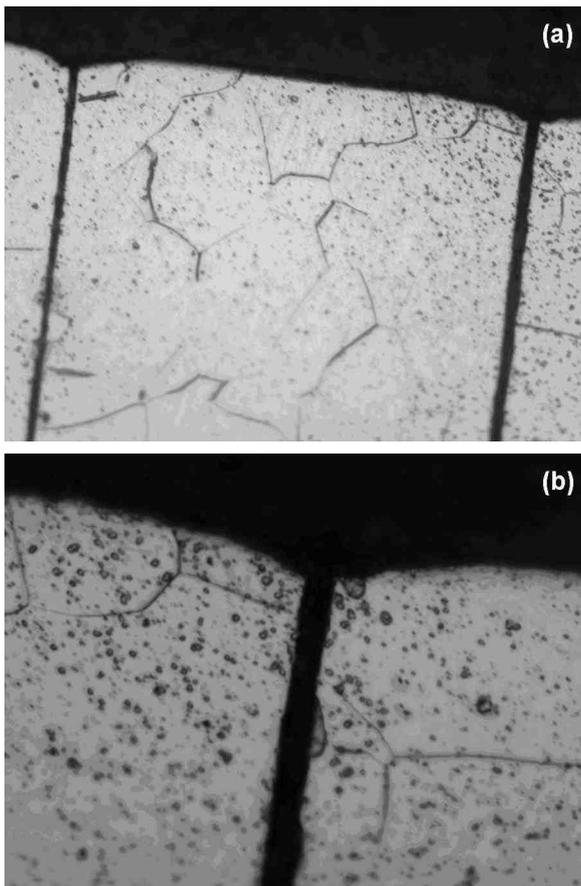
Figure 4—(a) OD surface electropolished - Cross section 400X; (b) OD surface electropolished - Cross section 1000X.
