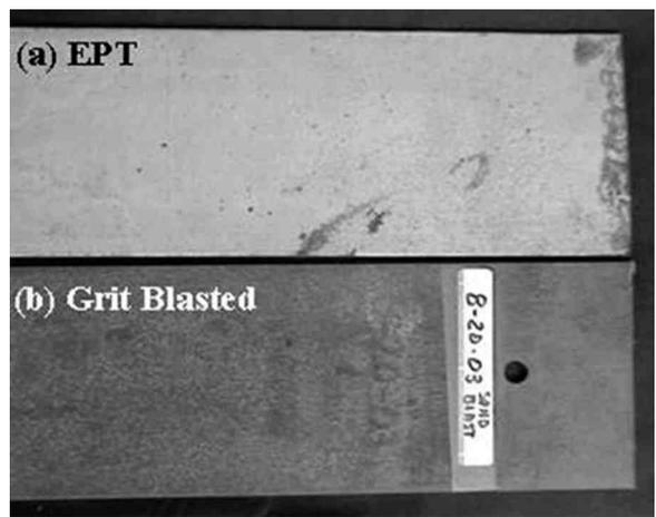
Figure 5—Level of rusting on steel strip, cleaned by (a) EPT and (b) grit blasting, after exposure for 6 months in the laboratory under a relative humidity of about 75%.
