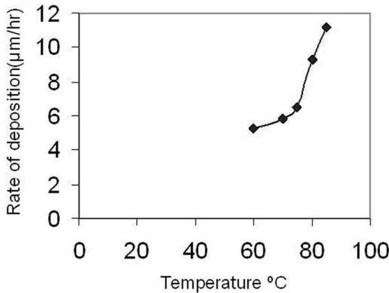
Figure 1—Effect of temperature on the deposition rate in the presence of TiO<sub>2</sub> particles (3.0 g/L at pH 4.0).
