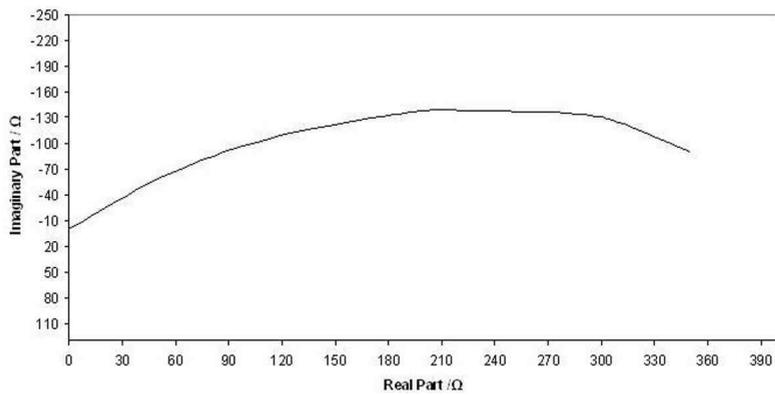
Figure 5(a)—Impedance curve (Nyquist plot) for an electroless-deposited specimen without heat treatment and  $\text{TiO}_2$  (Test conditions: potential:  $-0.511\text{ V}$ ; current:  $21.07\ \mu\text{A}$ ; temperature:  $-22.8^\circ\text{C} \pm 5.1^\circ\text{C}$  ( $-9.1^\circ\text{F} \pm 9.2^\circ\text{F}$ )).
