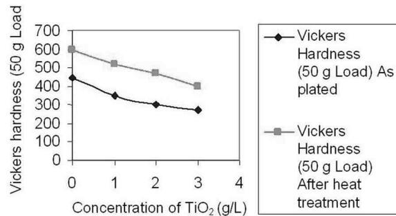
Figure 4—Effect of TiO<sub>2</sub> particle concentration on the coating hardness with respect to heat treatment.
