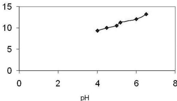
Figure 3—Effect of pH on the deposition rate in the presence of TiO<sub>2</sub> particles (3.0 g/L).
