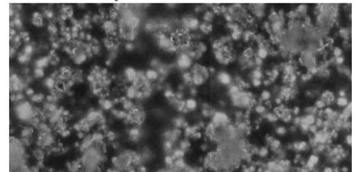
Figure 7—Microstructure of electroless-plated specimen from a bath with  $1.0\ \text{g/L TiO}_2$  (50X).
