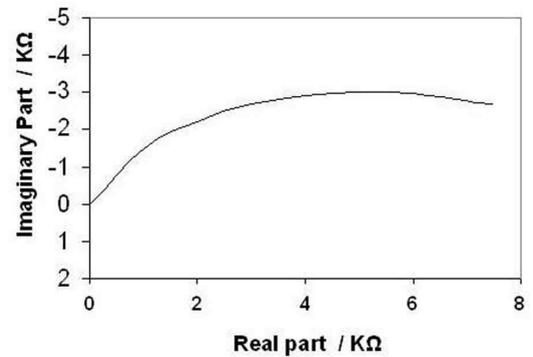
Figure 5(d)—Impedance curve (Nyquist plot) for an electroless-deposited specimen with heat treatment and  $3.0\ \text{g/L TiO}_2$  (Test conditions: potential:  $-0.338\text{ V}$ ; current:  $384.35\ \mu\text{A}$ ; temperature:  $-25^\circ\text{C} \pm 5.7^\circ\text{C}$  ( $-13.1^\circ\text{F} \pm 10.3^\circ\text{F}$ )).
