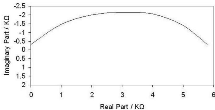
Figure 5(c)—Impedance curve (Nyquist plot) for an electroless-deposited specimen with heat treatment and  $2.0\ \text{g/L TiO}_2$  (Test conditions: potential:  $-0.405\text{ V}$ ; current:  $15.796\ \mu\text{A}$ ; temperature:  $-24.4^\circ\text{C} \pm 5.4^\circ\text{C}$  ( $-12.0^\circ\text{F} \pm 9.7^\circ\text{F}$ )).
