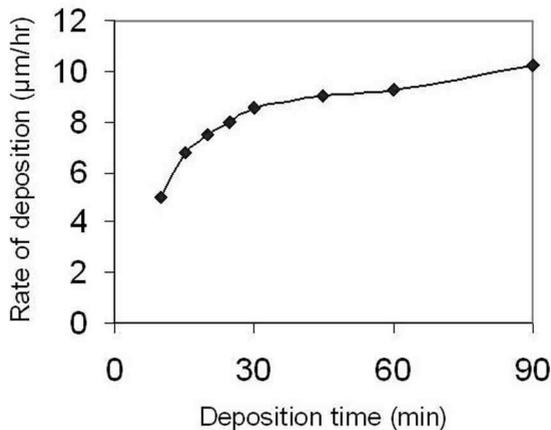
Figure 2—Effect of deposition rate with respect to deposition time in the presence of TiO<sub>2</sub> particles (3.0 g/L at pH 4.0 and a constant temperature of 80°C (176°F)).
