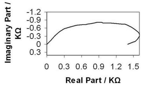
Figure 5(b)—Impedance curve (Nyquist plot) for an electroless-deposited specimen with heat treatment and  $1.0\ \text{g/L TiO}_2$  (Test conditions: potential:  $-0.42\text{ V}$ ; current:  $16.48\ \mu\text{A}$ ; temperature:  $-24.1^\circ\text{C} \pm 5.5^\circ\text{C}$  ( $-11.5^\circ\text{F} \pm 9.9^\circ\text{F}$ )).
