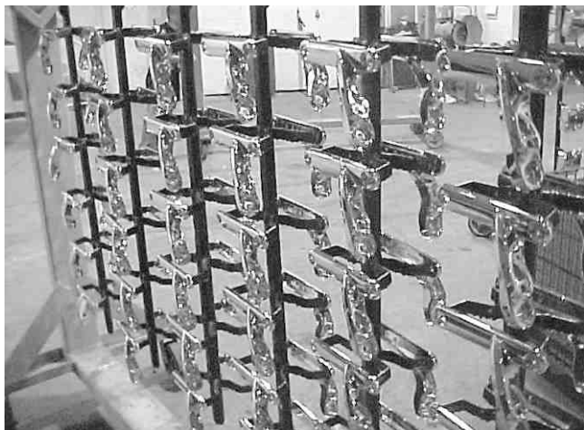
Large plating racks are used on Reliable Plating Works' automated lines.
