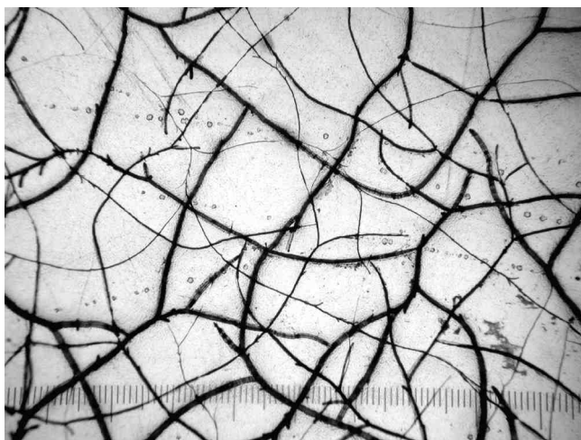
Shown (at 100X) is a crack pattern in the surface of a decorative chromium deposit, which can absorb traces of hexavalent chromium during plating.
