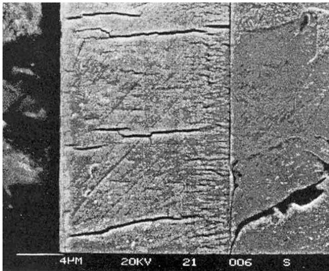
Figure 3—SEM micrograph of a Zn-Ni coating that contains more than 15% Ni. Poorly defined lamellar and microcracked structures, together with large continuous stress cracks, penetrate the electroplate (etched).
