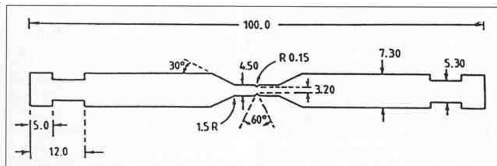
Figure 1—Dimensions of 3430 steel specimens used in tensile testing.
