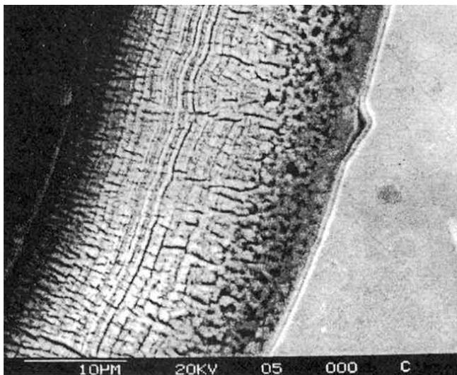
Figure 2—SEM micrograph of the etched Zn-Ni coating, showing a microcracked structure normal to the substrate extending through the plate. A well-defined lamellar structure normal to these cracks is apparent.
