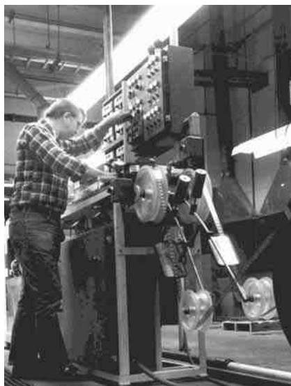
Figure 8—Spot plater for lead frames, providing continuous gold or silver spot plating of from four to forty lead frames. By means of stepping and repeating, ten to twelve spots were plated simultaneously through specially designed masking “shoes.” Four spot lines were required.
