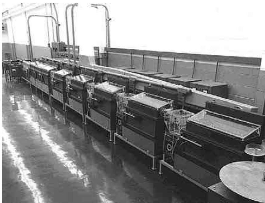
Figure 7—Continuous or reel-to-reel strip plater. Pre-formed or stamped strip sizes from 0.005” to 0.015” thick by 0.75” to 2.75” wide overall, or stripe plated with gold, silver, tin or solder over a nickel underplate. This and three similar lines were required.
