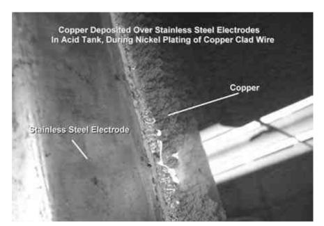
solution at low pH plates mostly gas, the efficiency (productivity) of the plating line is impacted.
