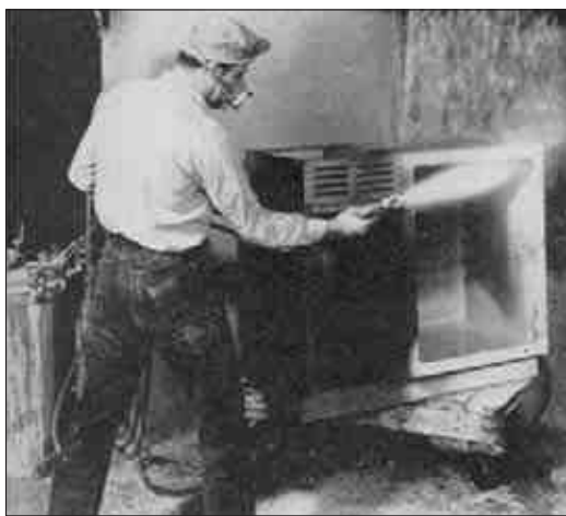
Paint, lacquer, enamel and other decorative coatings can be readily applied to electrogalvanized steel with assurance of long-term adhesion (Photograph courtesy of Weirton Steel Co.).
