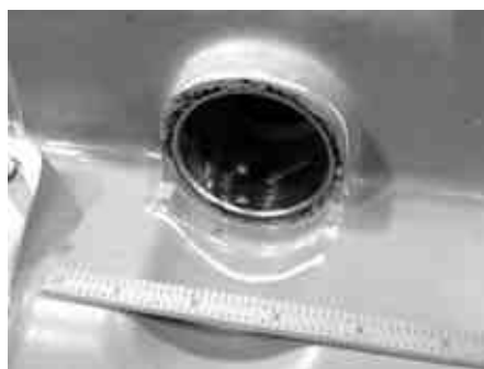
Figure 2—Corroded area on a magnesium transmission housing.
