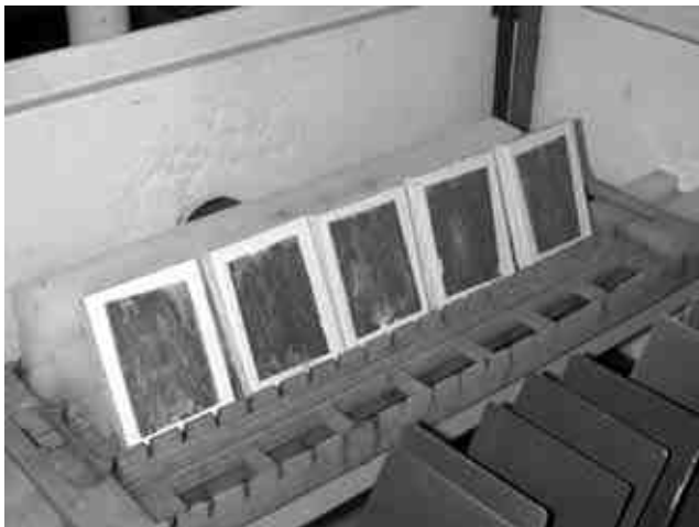
Figure 15—The panels sprayed using nitrogen gas after 8 hr of exposure.
