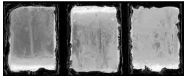
Figure 14—Cold spray CP-Al coated magnesium panels using helium gas after 336 hr of exposure in the salt fog chamber.
