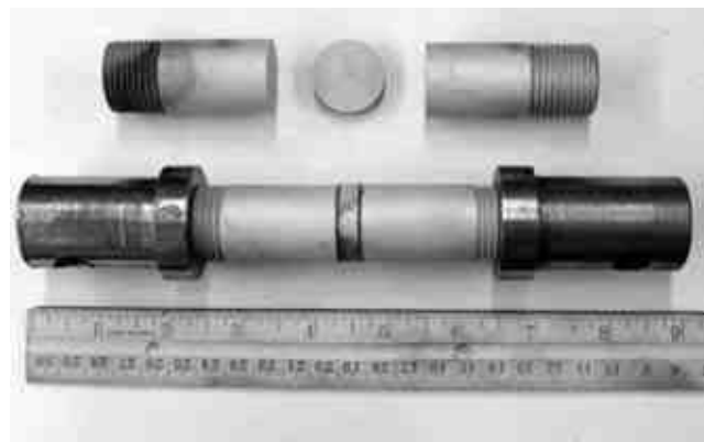
Figure 6—Bond bar adhesion test configuration.
