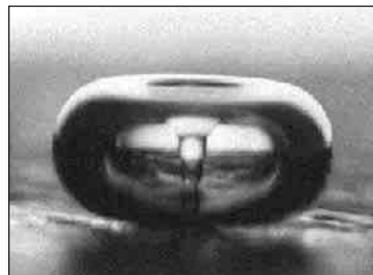
Figure 1—Bubble collapse at a solid surface (Photo by Prof. Crum, University of Seattle).
