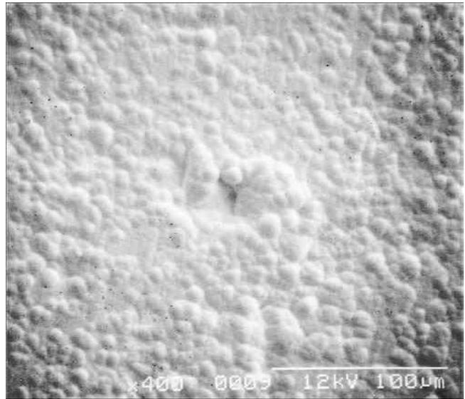
Figure 5—MC-21, double zincate activation, 1.0-hr Ni-P plate (400×).
