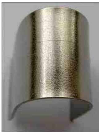
Figure 9—Ductility results for a 20- \mu m ternary alloy bent over a 12.5-mm mandrel.
