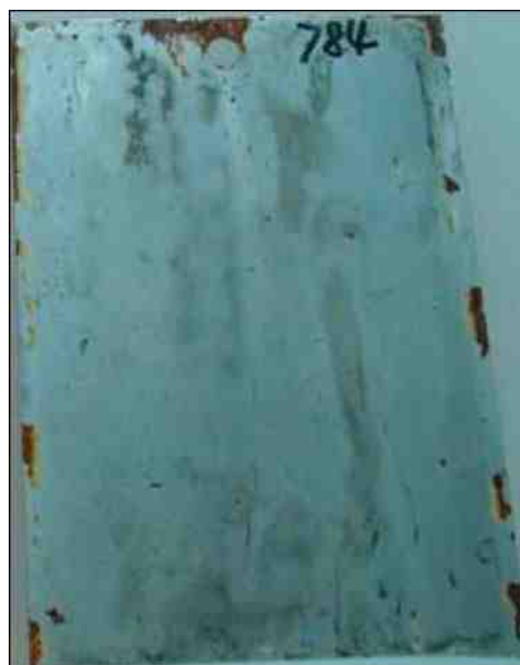
Figure 7—20- \mu\text{m} ternary alloy after 200 hr CASS.
