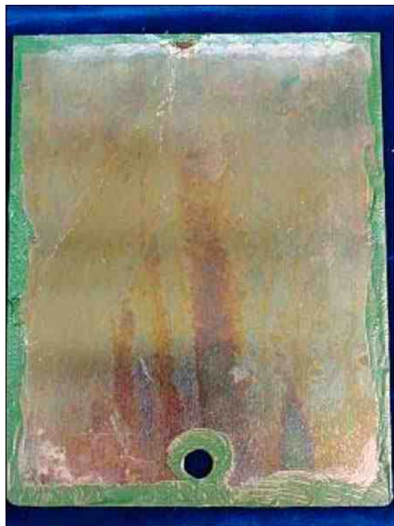
Figure 5—Aluminum panel plated with a 25- \mu\text{m} (1.0-mil) Ni-P-Sn deposit, after 2000 hr NSS.
