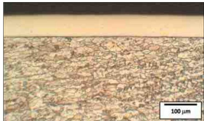
**Figure 11**—Cross-sectional photomicrograph of an XP coating over steel, after a 191°C bake for 24 hr. Note the absence of cracks.
