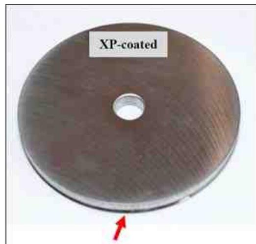
**Figure 12**—Photo of a commercial gravure wheel coated with the XP coating. The embossed letters on the outside diameter, which comprise the functional surface, can be seen on the bottom of the photograph (as highlighted by the arrow).
