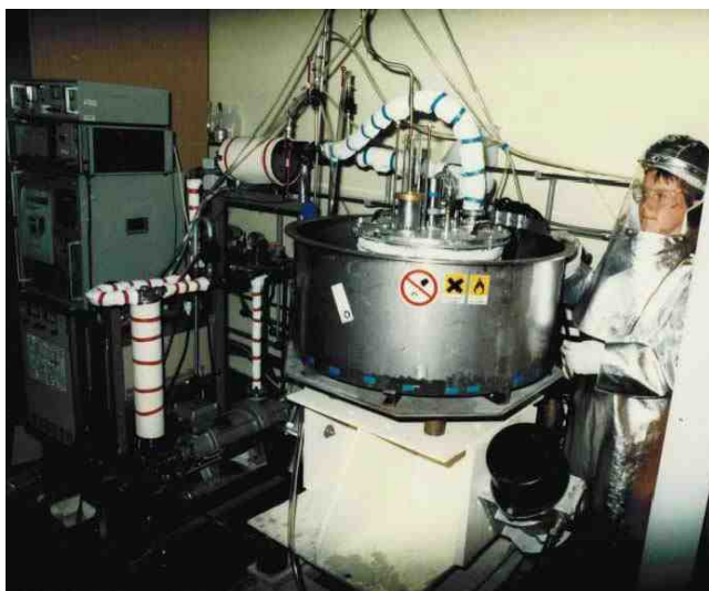
Figure 3 - Test apparatus for vibratory aluminum bulk plating without cooling equipment and storage tanks.
