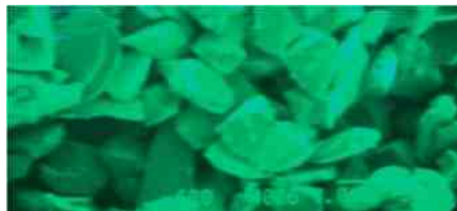
Figure 3 - SiC particles stirred 1 hr in a mid-phosphorus Ni-P bath, 93°C; no micro-nodules (600 \times ).
