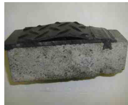
Figure 7 - V-Notch technique to anchor lining to concrete.
