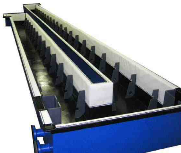
Figure 6 - Hard chromium plating tank with PTFE skirting.
