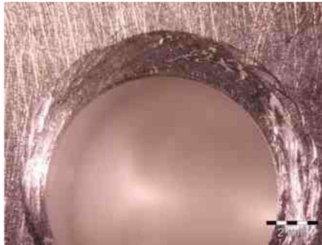
Figure 7 - Appearance of an ASU3 aluminum thrust plate after friction testing using the incorrect Zn/Ni plated screw ( \mu_g = 0.37 ).
