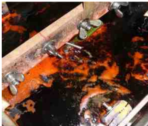
Figure 9 - Low-Foaming non-PFOS mist suppressant in a hard chromium plating tank.
