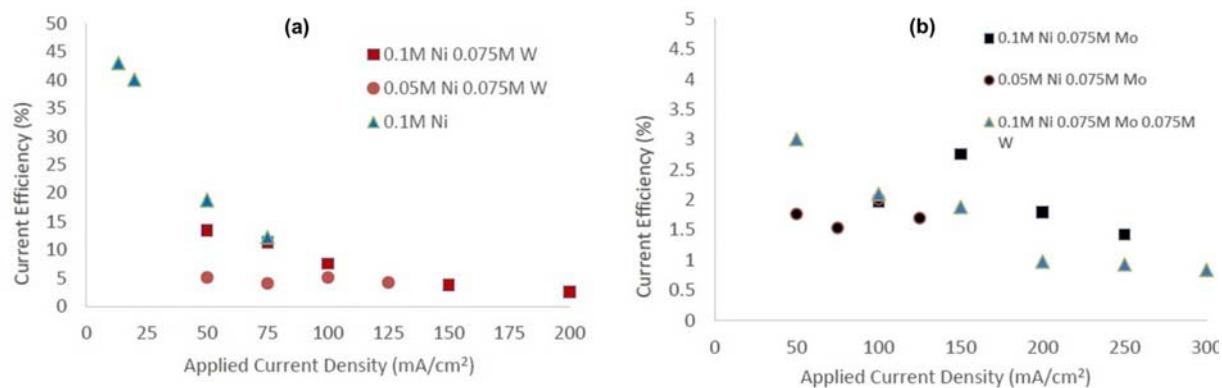
Figure 3 - Current efficiency in (a) electrolytes with tungstate ions, and (b) where molybdate is present.
