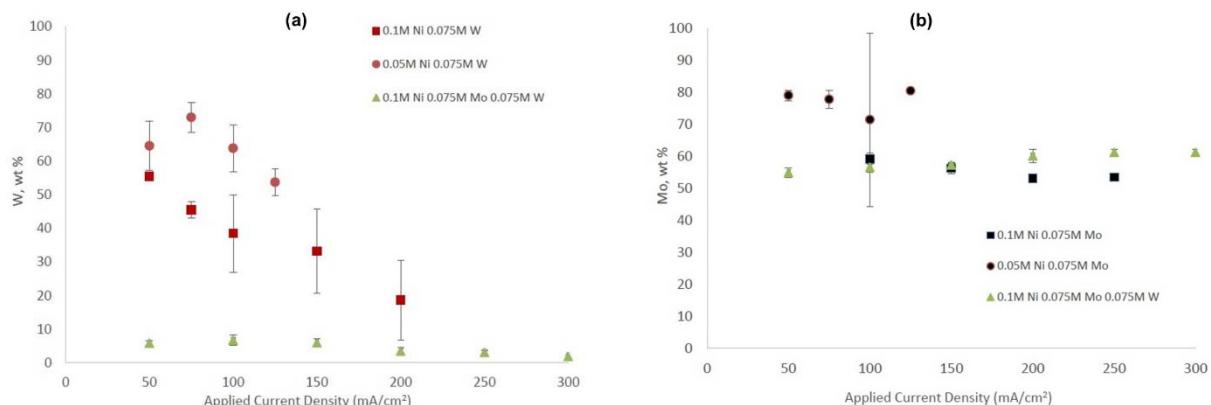
Figure 2 - (a) Tungsten composition in Ni-W and Ni-Mo-W deposits, and (b) molybdenum composition in Ni-Mo and Ni-Mo-W deposits produced at different applied current densities.
