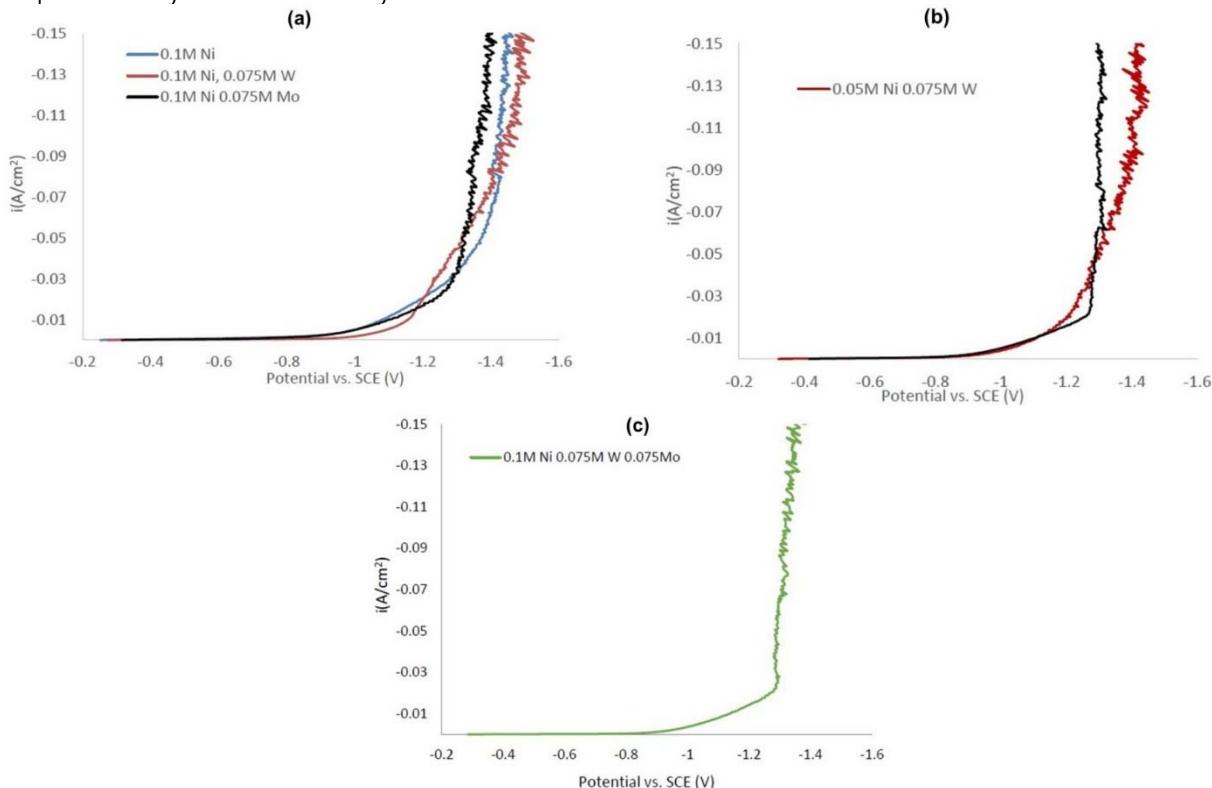
**Figure 1** - Polarization curves with different concentrations of (a) binary electrolytes using 0.1M nickel are combined with electrolytes containing either 0.075M tungstate or molybdate, (b) binary electrolytes using 0.05M nickel with electrolytes containing either 0.075M tungstate or molybdate and (c) the ternary Ni-W-Mo system.
