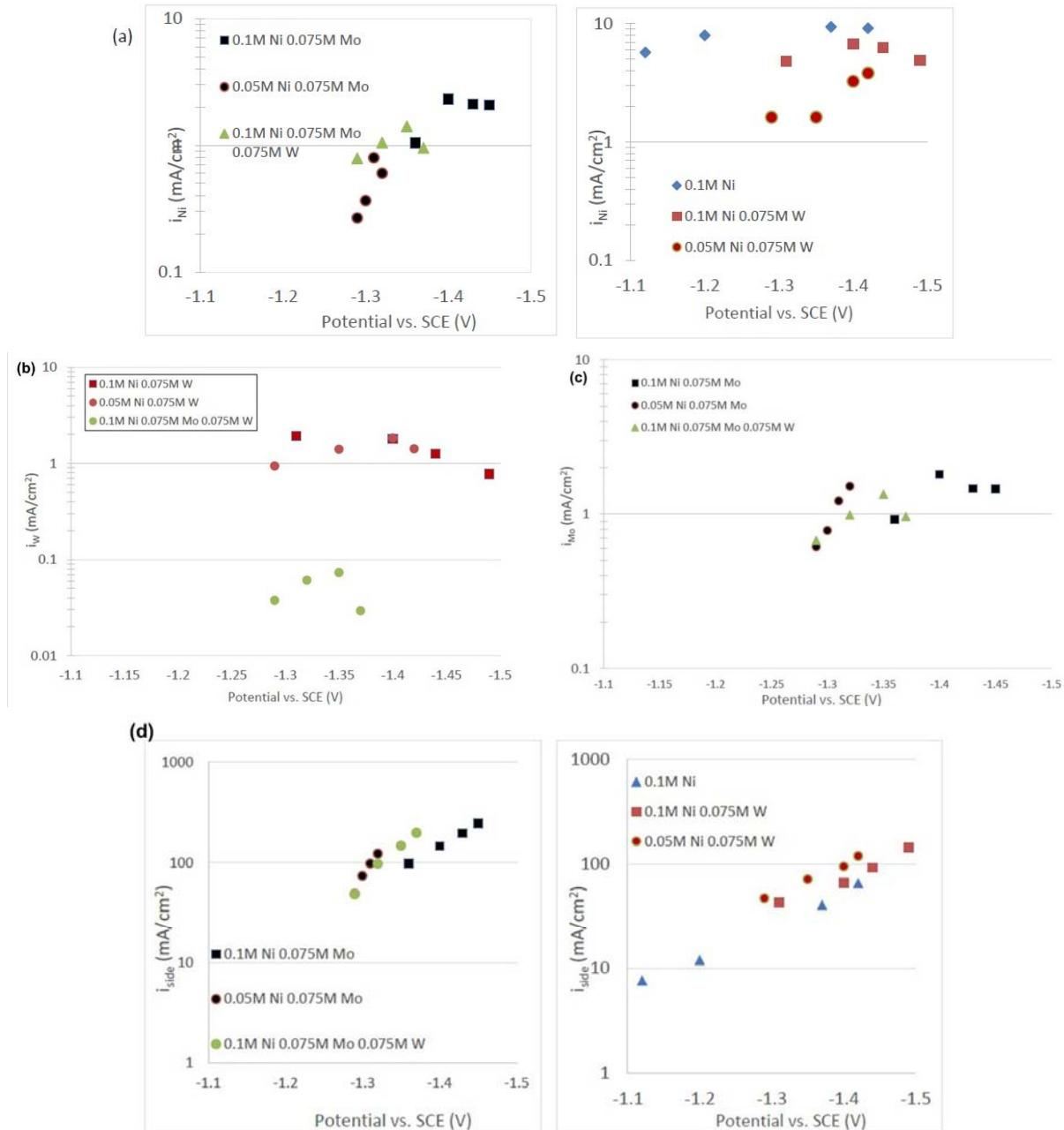
**Figure 4** - Partial current density of (a) nickel, in the Ni-Mo and Ni-Mo-W electrolytes (left) and Ni-W and elemental nickel (right), (b) tungsten, (c) molybdenum and (d) side reaction in the Ni-Mo and Ni-Mo-W electrolytes (left) and Ni-W and elemental nickel (right).
