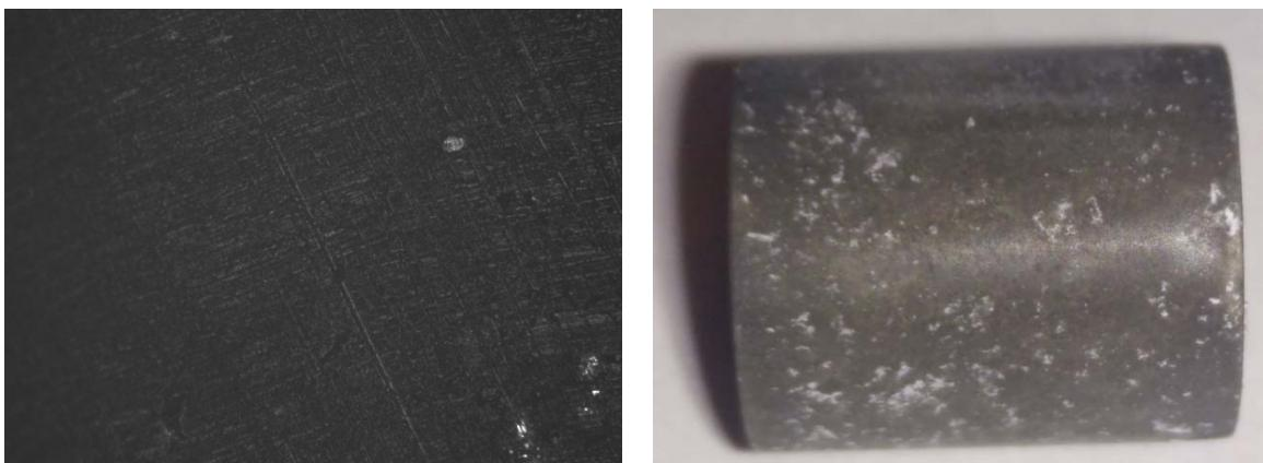
Figure 5 - Optical image and photograph of 0.1M Ni deposit using an applied current density of 50 mA/cm<sup>2</sup>.
