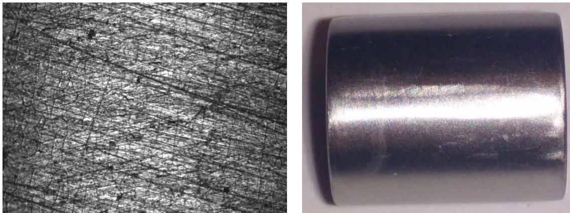
Figure 6 -Optical image and photograph of 0.1M Ni - 0.075M W deposit using an applied current density of 50 mA/cm<sup>2</sup>.
