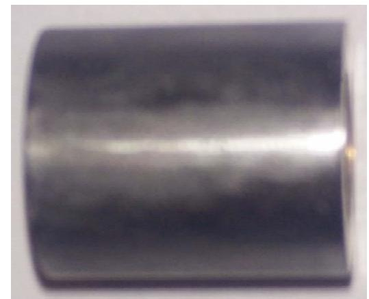
Figure 8 - Optical image and photograph of 0.1M Ni-0.075M Mo-0.075M W deposit using an applied current density of (a) 100 mA/cm<sup>2</sup> and (b) 250 mA/cm<sup>2</sup>.
