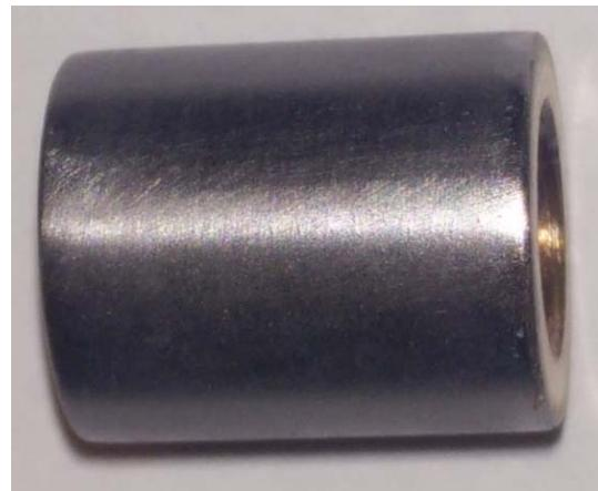
Figure 7 - Optical image and photograph of 0.1M Ni - 0.075M Mo deposit using an applied current density of 200 mA/cm<sup>2</sup>.
