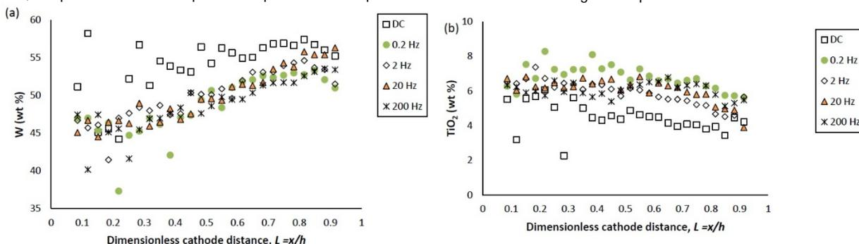
**Figure 1** - Ni-W- $TiO_2$  deposit composition of (a) tungsten and (b)  $TiO_2$  (wt%) under DC and PC (with variable pulse frequency) conditions, with respect to a dimensionless length  $L$  representing lower and higher current densities with smaller and larger values, respectively.
