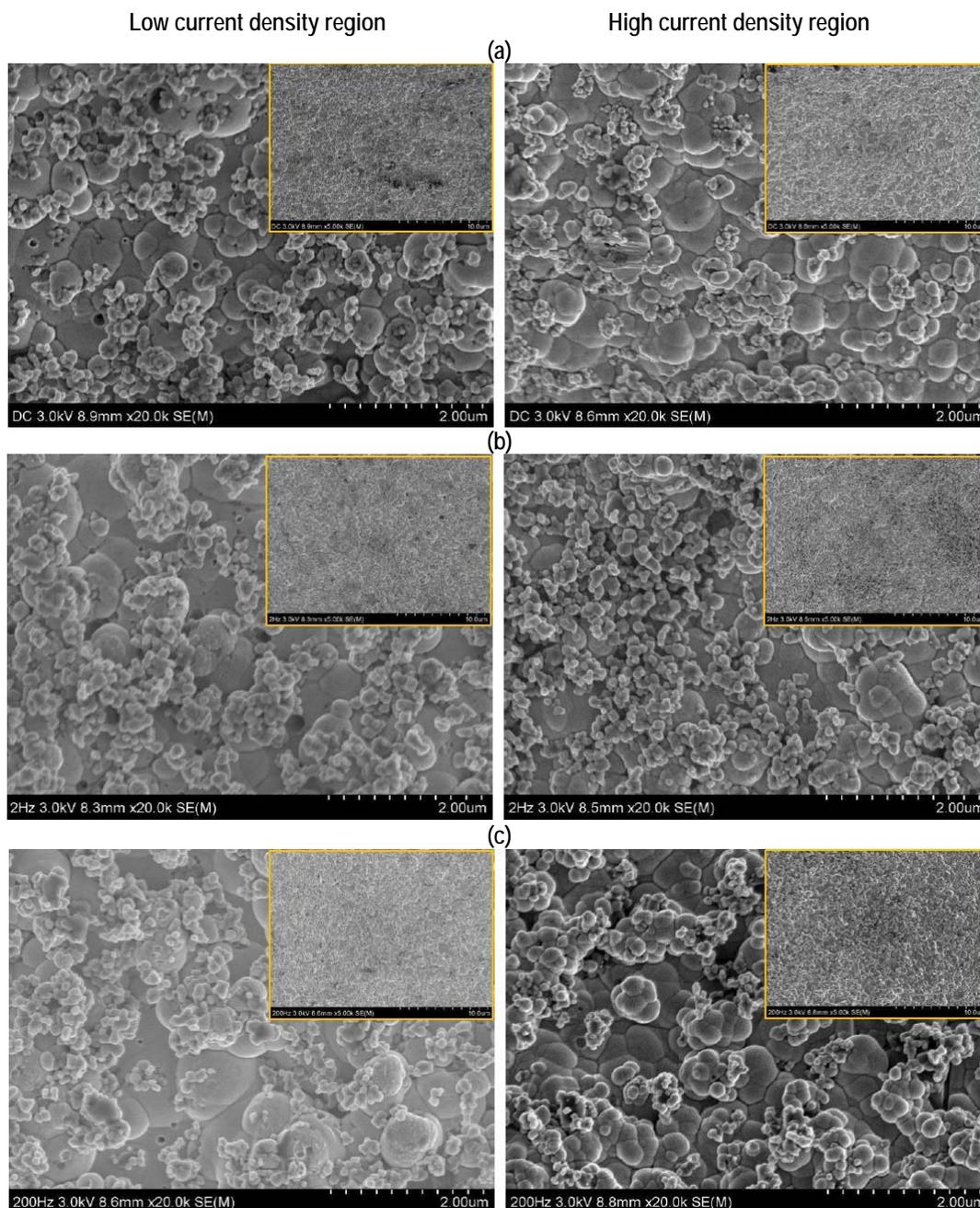
**Figure 3** - SEM images of Ni-W-TiO<sub>2</sub> deposits plated with (a) DC, (b) PC with the frequency of 2 Hz and (c) PC with the frequency of 200 Hz, in low current density (left) and high current density (right) regions, at low (5K, inset, upper right) and high (20K) magnifications.
