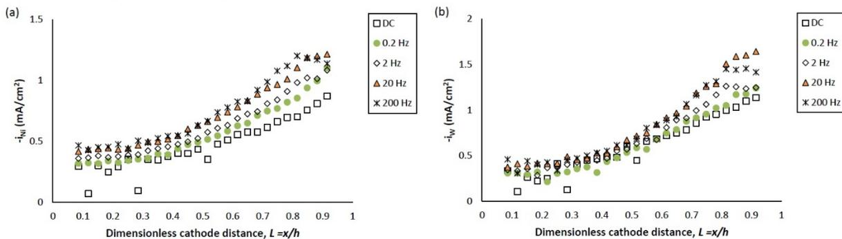
**Figure 2** - Partial current density of (a) nickel and (b) tungsten under DC and PC (with variable pulse frequency) condition, with respect to a dimensionless length  $L$  representing lower and higher current densities with smaller and larger values, respectively.
