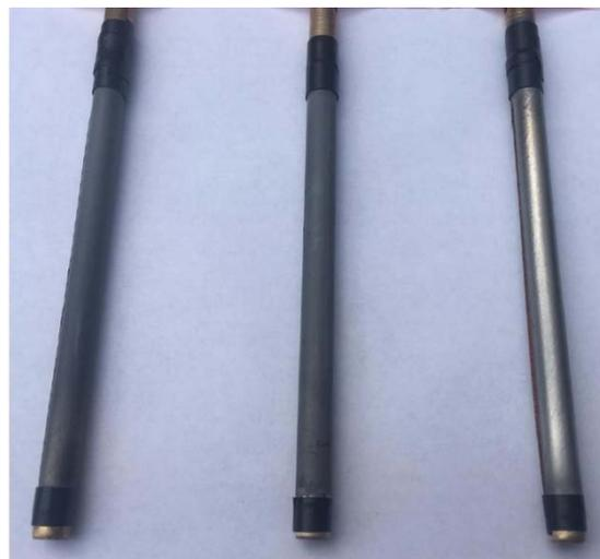
**Figure 4** - Photographs of Ni-W-TiO<sub>2</sub> composite coatings plated with DC with no BD, PC with no BD, PC with 5mM BD (from left to right) on the rotating Hull cell.
