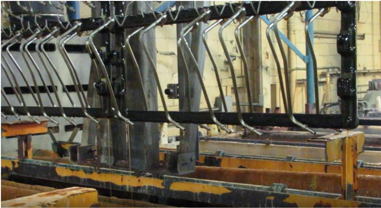
**Figure H-4. Dragout Still Draining Just Prior to Rinsing**
