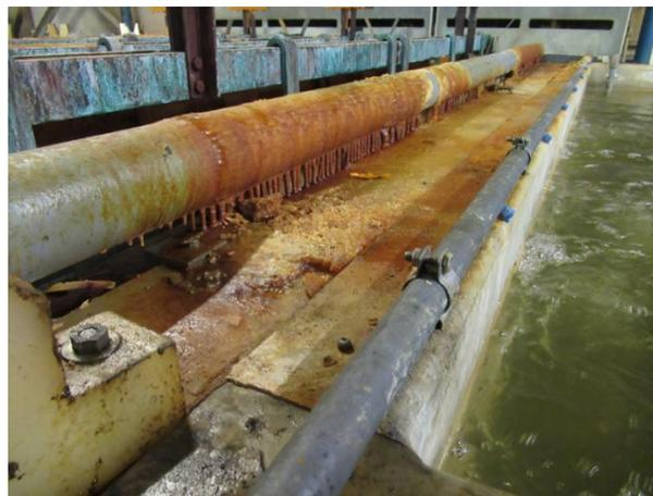
*Figure H-7. Buildup of Chemicals Occurs Between Tanks Due to Lack of Drip/Drain Board*
