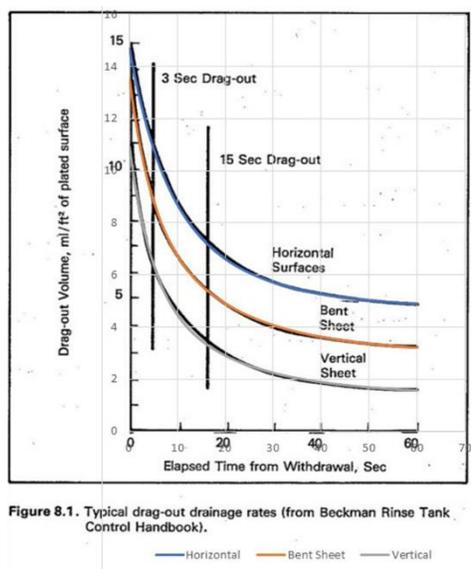
Figure 8.1. Typical drag-out drainage rates (from Beckman Rinse Tank Control Handbook).
