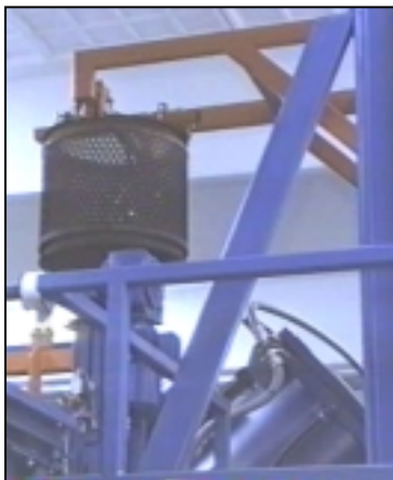
Figure 3. A centrifuge basket under automatic transportation with fasteners before the chromating process step.
