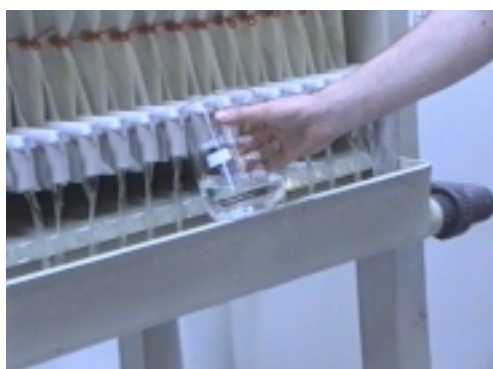
Figure 6. Two filter presses are used to make it possible to separate chromium and non chromium containing sludge. All the wastewater is filtrated and finally treated by an selective ion exchange to eliminate zinc and chromium. Typical values of Zn and Cr is usually between 0.00 and 0.25 ppm.
