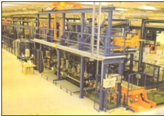
Figure 2. A view over the zinc plating line with integrated centrifuges in the post-treatment processes. The centrifuges can be seen in the front of the picture.
