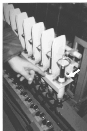
Figure 3 – White arrow shows where the system of ring and clasp type components are applied on a textile machine
